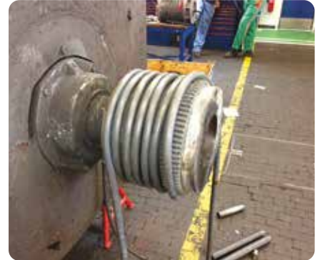
Heating a coupling for dismounting
