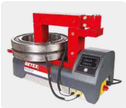
Recommended horizontal heating position
