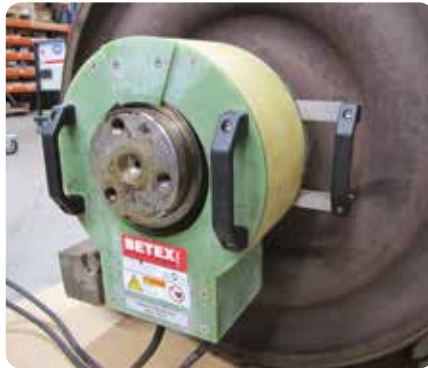
Heating bearing rings for dismounting
