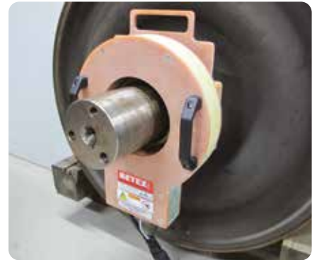
Heating labyrinth rings for dismounting
