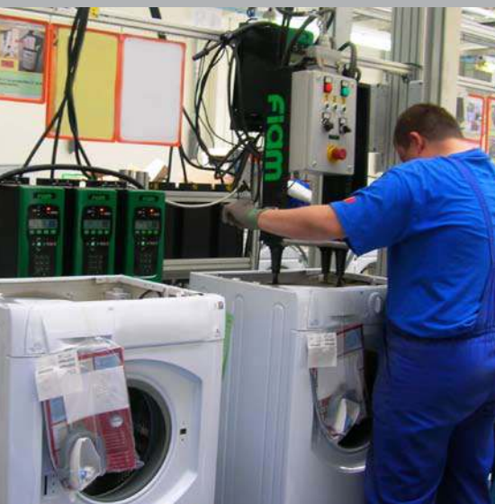
Example of multispindle tightening unit, manufactured for appliance components , equipped with computerized controlled electric nutrunner motors
