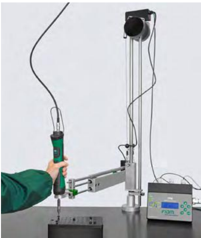
Cartesian arm with a position monitoring device.
