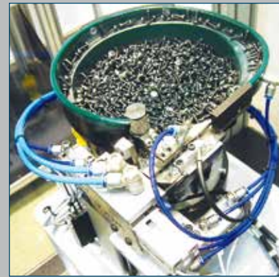
The photo shows an application of Fiam ALC feeder
