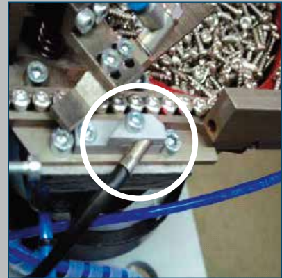
The photo shows an application of a Fiam overload sensor with optical fibre
