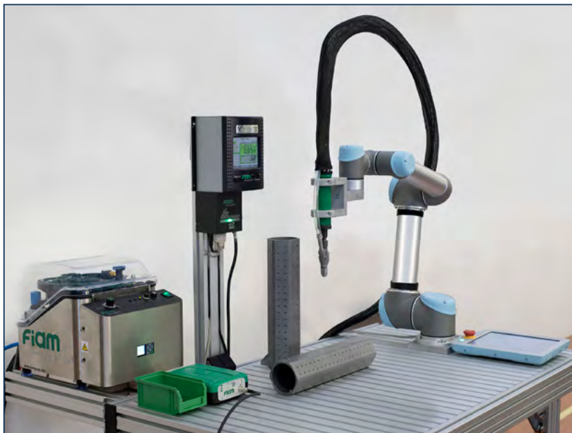
Example of MCA with collaborative robot
