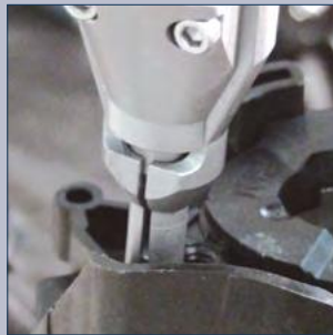
Examples of special heads with friction jaws to access to deep tightening points, behind shoulders or for entering very narrow holes
