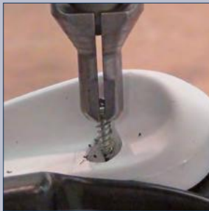
Examples of special heads with friction jaws to access to deep tightening points, behind shoulders or for entering very narrow holes
